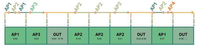
Fig. 1. Discretization of irregular connection events into one-minute intervals. The original AP connection timeline (top) and the resulting discretized sequence (bottom) are shown.
